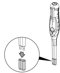
2. After every measurement put the protective cap back on the measuring electrodes.
